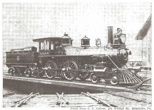
SMALL cylinders and low boiler pressure put very little strain on old-time axles and pins. This handsome New Orleans & North Western (MoP) eight-wheeler was originally built for the Erie and remodelled in that road's Meadville (Pa.) shops
