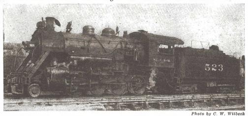
ARCH separating footboard segments distinguishes engines used in switching
