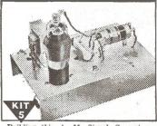
Building this A. M. Signal Generator gives you more valuable experience. It provides amplitude-modulated signals for many tests and experiments.
