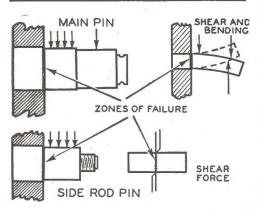
exerted on the pistons and passed back to the main pin. If the drivers have an outside diameter of seventy-five inches there will be 268 revolutions for every mile traveled. Double that figure for the number of strokes and the wonder is that there is anything left of the pins and axles after a hundred thousand miles of fast running.
